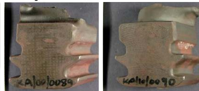
Analysis of broken blades
