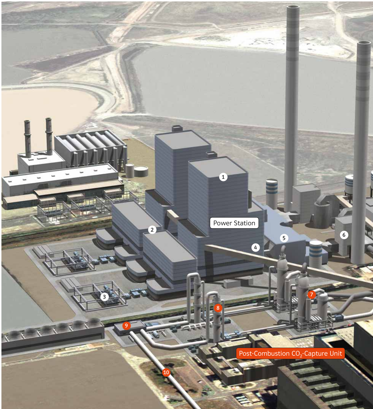
Engineering design: a 3-D computer-generated image of a CCS demonstration plant on a full-scale coal-fired power station.
