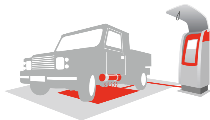
With suitably equipped parking spaces, an electric car can be charged without the need for cables.
