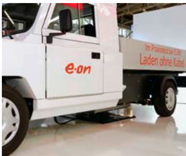
With suitably equipped parking spaces, an electric car can be charged without the need for cables.
