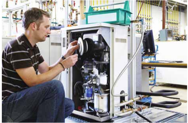
Micro CHP in testing operation
